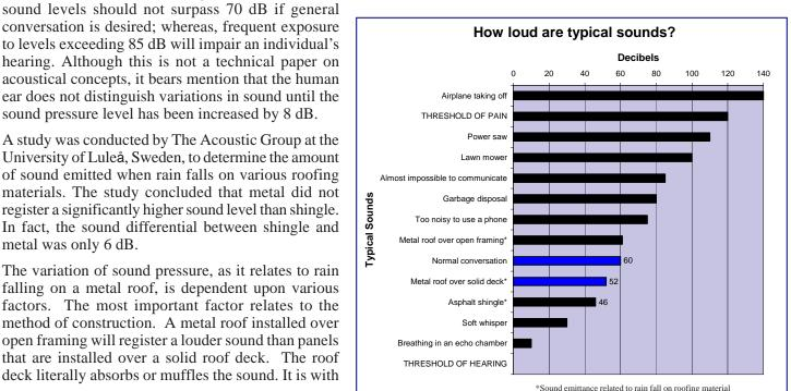
A study was conducted by The Acoustic Group at the University of Luleå, Sweden, to determine the amount of sound emitted when rain falls on various roofing materials. The study concluded that metal did not register a significantly higher sound level than shingle. In fact, the sound differential between shingle and metal was only 6 dB.
